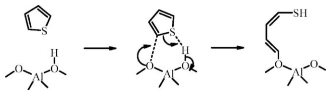
Scheme 1. Reaction mechanisms in the cracking of thiophenic rings catalyzed by acidic zeolites.
